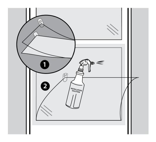
Every piece of ComforTech™ window film has a clear polypropylene liner protecting the film's adhesive.
